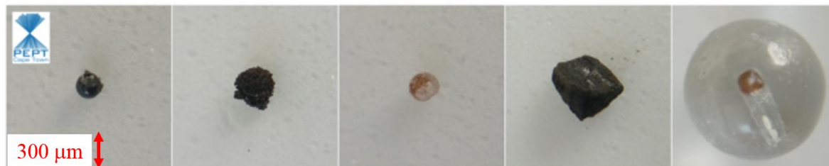
Figure 2. A selection of PEPT Cape Town tracer particles from left to right: moulded, density modified, mineral coating, silica coating, coal particle, glass bead with ion-exchange inset. The images have a global scale with the tracer on the far left approximately 300 \mu\text{m} in diameter, up to 1 mm diameter on the far right.
